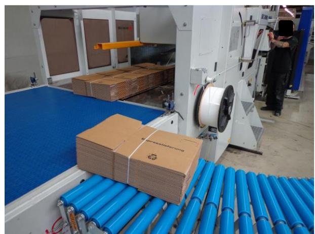
The closely spaced spherical ball table ensures that the products are suitably and carefully handled to eliminate any possible damage. This feature also enables very small products to be securely and simply handled in the system after squaring and strapping. The bundles can be positioned anywhere on the table for easy removal by the line operator, as table safety guarding or protection is not normally required.
