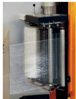
Solution with Power-Pre-Stretch: Pre-stretching of the film up to 300% (option) – optimum utilization of the film!
