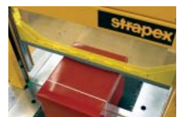
Hold down device for compressing loose packages
