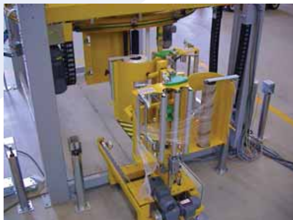
An automatic film reel changer is an optional feature for the Octopus. A two reel changer is pictured here (RCSII).
